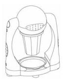
To insert or remove the jar, turn the device into the start position (jar points downwards).
